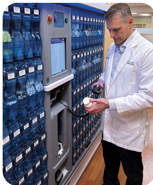
Matt Gerig, RPh, FCHC Retail Pharmacy Director, scans a medication's bar code with the dispensing robot.
